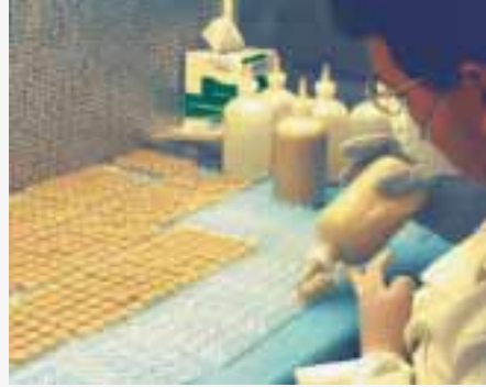
2. Dispensing the mixed diet into cells (manual for now, but to be automated later).
